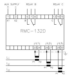
The auxiliary supply connection may be protected by a 2A fuse.
