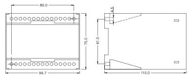
The RMC-132D is designed for panel mounting, being mounted on a 35 mm DIN rail, or by means of two 4-mm screws.
